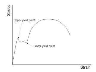
Product that does not exhibit these lines when formed is usually called non-fluting and is likely related to tension-leveling and/or temper passing practices after annealing.
